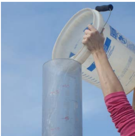
Figure 9. Filling infiltrometer with water
